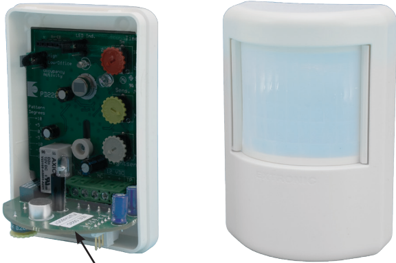
PD-22LF circuit board mounted in IR detector PD-2200.
