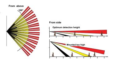
The detector should be installed at a height and to be directed against the part of the man who radiates the most energy (trunk). Suitable installation height is usually 1.6 to 1.9 m.
