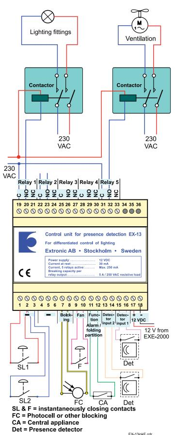
Inputs 1 - 4 (contact units 1-6): Instantaneously closing contacts which switch the lighting on and off are connected to these.
