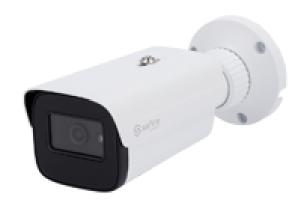
Safire Smart Range I1 with Advanced Artificial Intelligence Bullet IP camera 1/3" Progressive Scan CMOS 4 Megapixel (2592x1520) 3.6 mm Lens 0 Lux IR Range 50 m Compression H.265+ / H.264+ WDR 3DNR Audio Advanced Artificial Intelligence: human, vehicle and non-motorized vehicle detection Facial Capture Video metadata Human, vehicle and non-motorized vehicle counts WEB, CMS, Smartphone and NVR interface **ONVIF** Compatible PoE (IEEE802.3af) Weatherproof IP67
